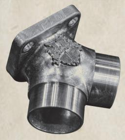
Compared to the OEM manifold, the port diameter  $(35\pi)$  is larger, improving the intake and flow rate of the air-fuel mixture from the carburetor, resulting in significantly improved response. \*Proven through chassis dynamometer testing.
